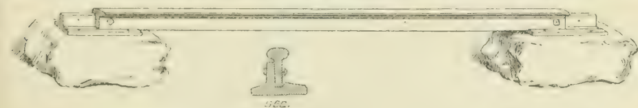
Fig. 24. EDGE RAILS, LAWSON COLLIERY, NEW CASTLE-ON-TYNE. (1797.) [From model in the U. S. National Museum.]
