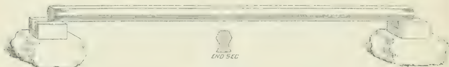
Fig. 25. WYATT'S HEXAGONAL RAIL, BANGOR, NORTH WALES. (1802.) (From model in the U. S. National Museum.)
