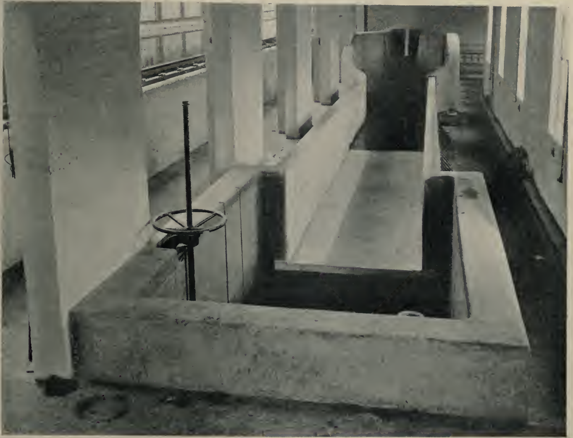
FIG. 3.—National Physical Laboratory Experimental Tank. The small tank for still or flowing water experiments.
