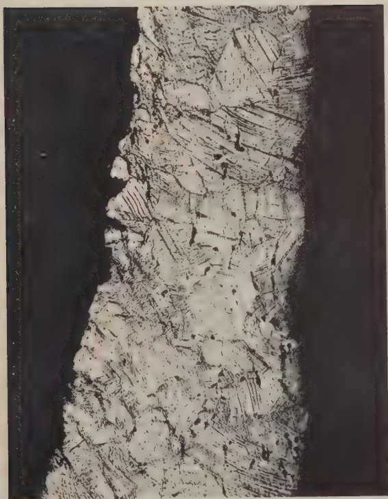
FIG. 34. Piece of old brass of the 17th Century used for comparison. Etched section showing inclusions (dark spots). Magnification 200.
