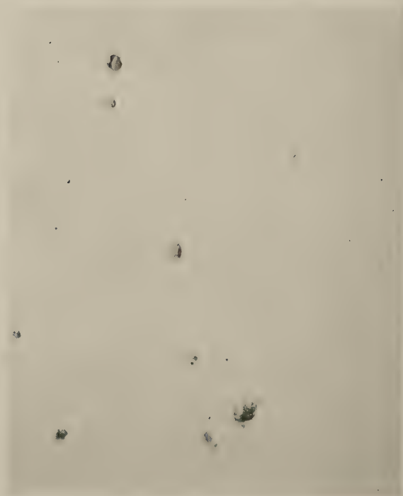
FIG. 32. Appearance of inclusions at high magnification, 1000.
