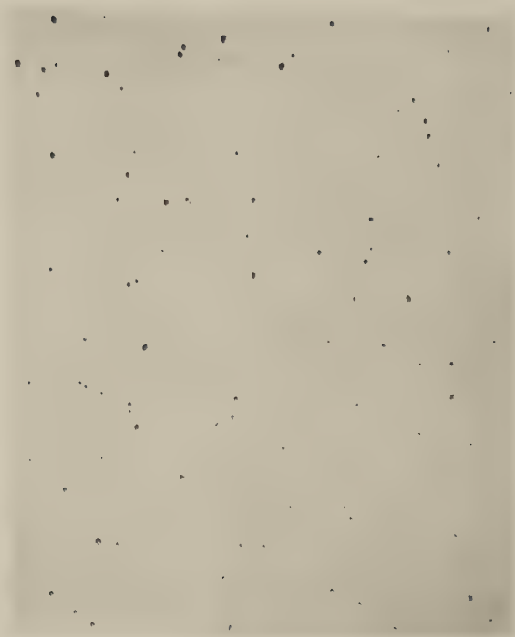
FIG. 31. Inclusions (dark spots) in another polished section of the Plate. Magnification 200.
