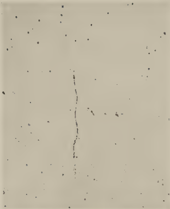
FIG. 35. Globular inclusions in the Plate following a fine, wavy crack. Magnification 200.
