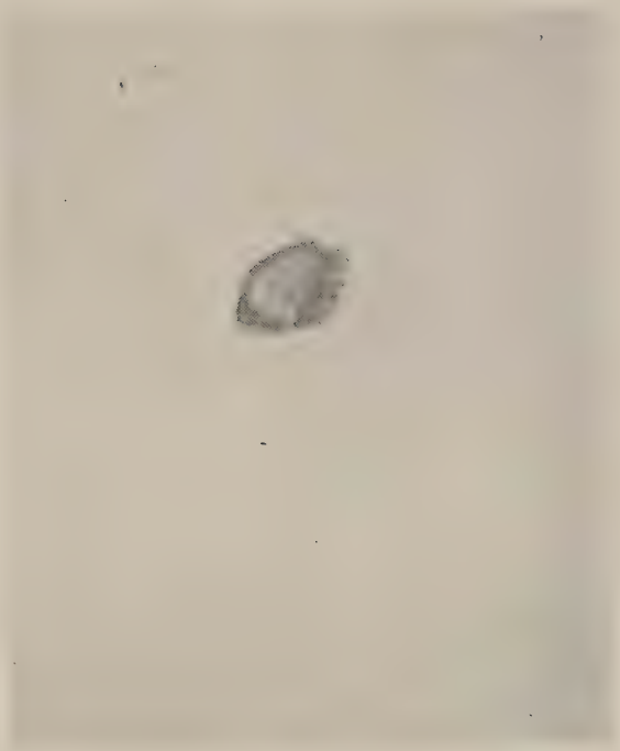
FIG. 33. A large, transparent inclusion (dark area); probably a grain of quartz sand. Magnification 750.
