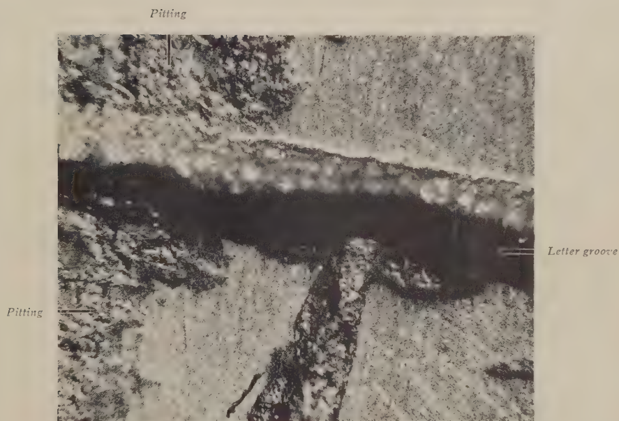
FIG. 10. Pitting in the face surface of the Plate. Magnification 30.
