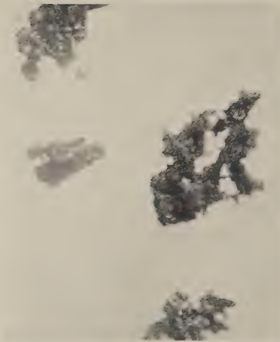
FIG. 23. Particles of patina before heating. Predominant color, black. Magnification 75.
