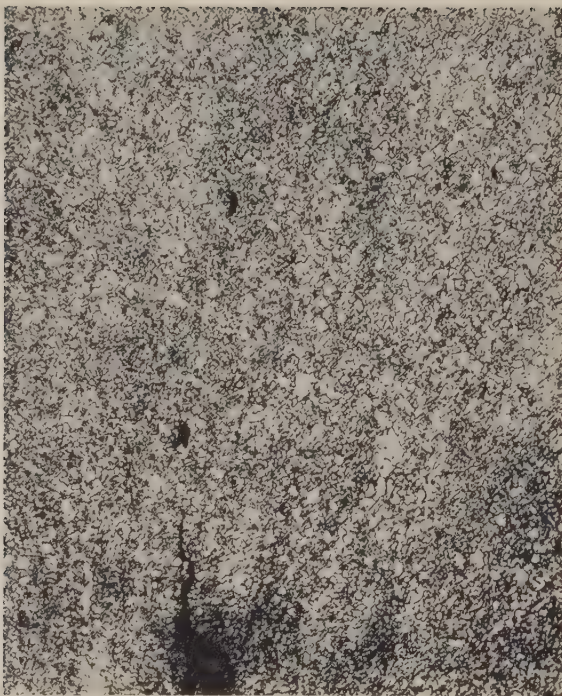
FIG. 47. Microstructure of an area of a section of the Plate showing small grains only. Etched with ammonium persulfate. Magnification 200.
