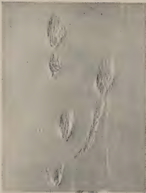
FIG. 17. Indentations made by the authors on a piece of modern brass with stone ax, simulating those shown in Figs. 6 and 15. Magnification 3\frac{1}{2} .
