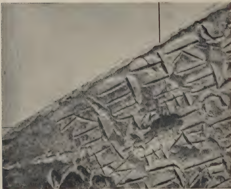
FIG. 4. Burr (X) at edge of Plate Magnification 3.5 g
