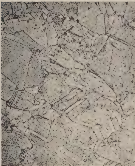
FIG. 45. Microstructure of another section of the Plate showing large and small grains. Etched with ammonium persulfate. Magnification 200.
