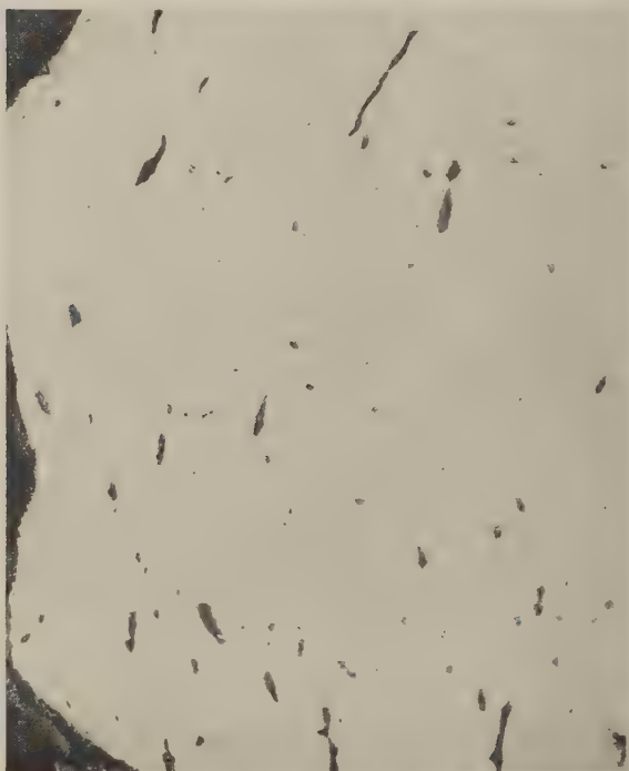
FIG. 36. Elongated inclusions in an old brass used for comparison study. Inclusions are not in parallel arrangement. Magnification 200.
