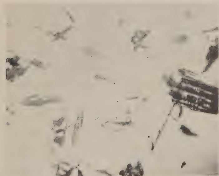
FIG. 26. Particles of patina from the coin groove of the Plate. Some particles show a fibrous structure. Magnification 100.
